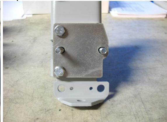
Slide the smaller aluminum spacer over the engine mounting bolts and attach to your engine.
