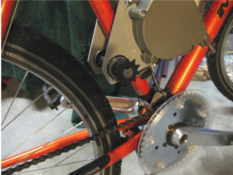
Check alignment of the right side sprocket and outer chainring. You can take a measurement using the seat post as a reference.
