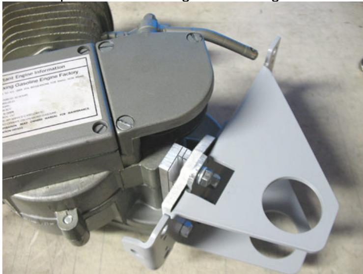
Start with the spacer stack up as shown below, use the 1/4 inch thick spacer and the two 1/8 inch T spacers.
