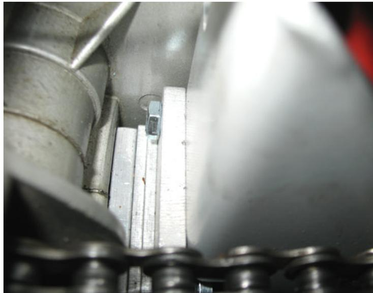
Due to the variations in the castings and hole locations of the different engines some modification to the mount may be necessary. Verify fit of the upper mounting hole.
