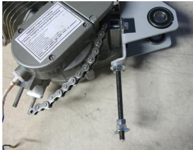
Sandwich the lower tab on the rear mount with two of the nuts. Use a washer on the bottom side. Do not tighten these down yet. The lower two nuts should also be threaded onto the rod at this time.
