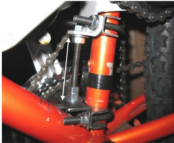
Add 1.5 inches to your measurement and cut the adjuster rod to that length
