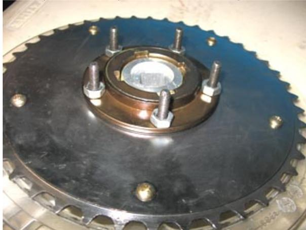
8. Then slide the smaller sprocket onto the bolts with the bevel side of the teeth facing the other chainring. The goal here is to separate the chains as much as possible.
