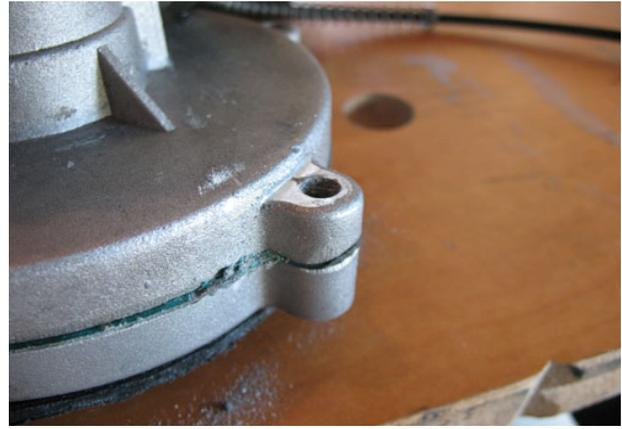
Flatten the back side of the upper rear clutch cover mount as shown above.
