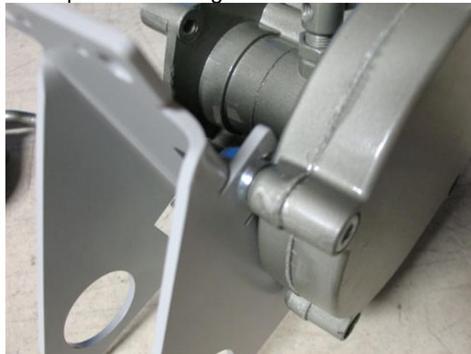
2. Install one of the two supplied cap screws. Which one to use will depend on your engine. Some engines have wider clutch covers. You will need enough of the end of the bolt protruding past the mount to install the supplied lock nut. Install the nut at this time but do not tighten it down. This will be done after final chain adjustment.
