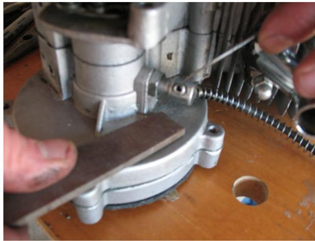
Remove any casting bump that will keep mount from mounting flush to the back of the clutch case.
