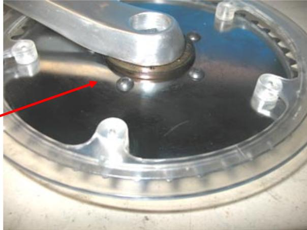
7. Next place the 5 spacers (6mm nuts) over the bolts up to the freewheel.
