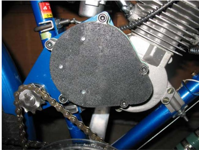
6. Install the chain guard by screwing it to the clutch plate.
