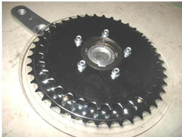
10. Tighten the chainring assembly with the 5 locknuts and washers. Be sure that the bolts are tight against the outer chainring before installing the locknuts.
