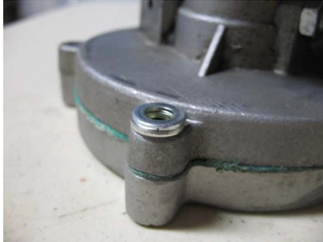
1. Add the correct number of 6mm washers to get the mount to sit flat against the back of the clutch case. Note there are thick ones and thin ones, use whatever combination works best so that the plate sits flat against the clutch case.
