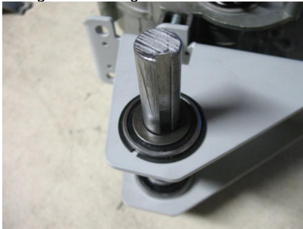
3. Install the larger sprocket onto the shaft after placing one of the thin shim washers and then two of the thicker spacer washers on. The sprocket hub should be toward the outside.
