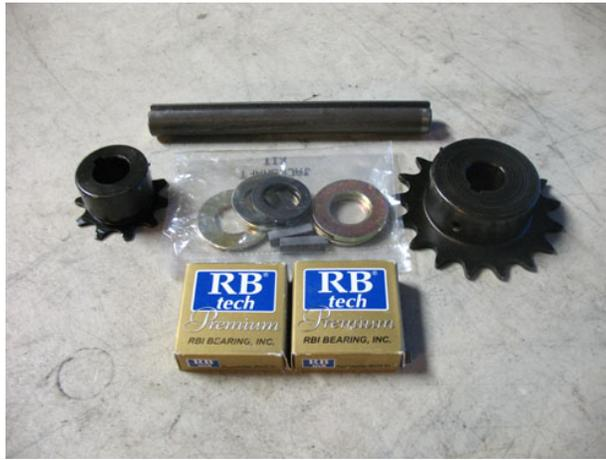
1. Install the bearings into the opening on the rear mounts. The lock rings on the bearings should be to the outside of both plates. Some sanding may be required to get the bearings to fit. They should fit snug but be able to be inserted by hand.
