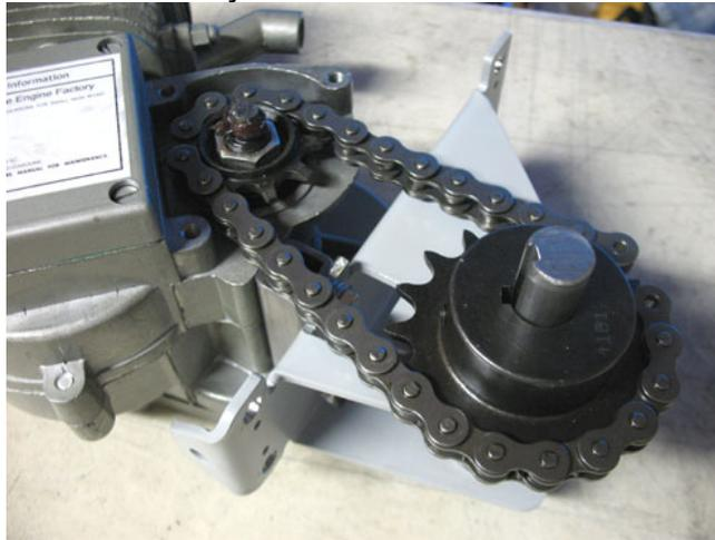
Remove the left side sprocket and shaft.
