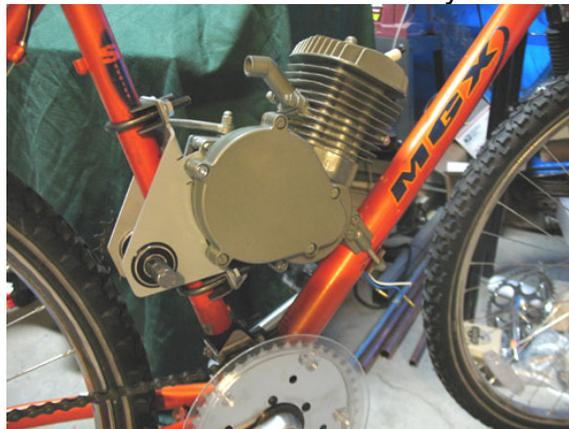
Measure the distance between the lower chain adjuster bracket and the tab on the lower part of the rear mount.
