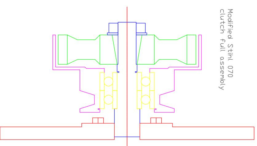
Stihl 070 clutch shoes I use is having push lock mechanism. Other model might have keyway, threaded, etc.
